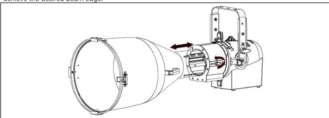
Step 2. Once the luminaire is focused, tighten the locking bolt.
