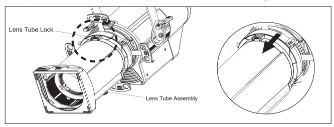
Step 2. Lift lens tube assembly up and away from light engine assembly.
